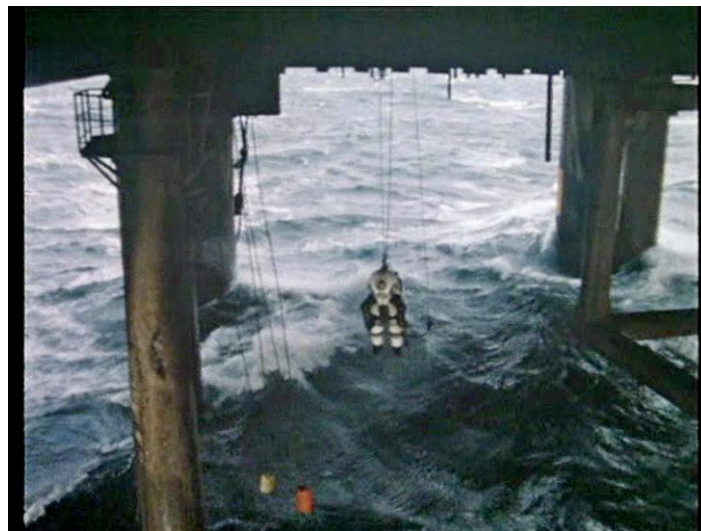
Image 1 - Deploying JIM from oil rig
